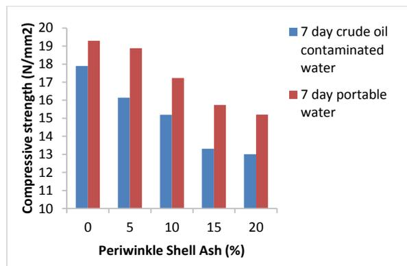
**Fig. 1:** Variation of compressive strength of periwinkle shell ash blended cement concrete cubes with periwinkle shell ash content cured for 7 days in portable water and crude oil contaminated water
