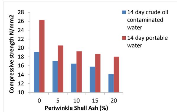
**Fig. 2:** Variation of compressive strength of periwinkle shell ash blended cement concrete cubes with periwinkle shell ash content cured for 14 days in portable water and crude oil contaminated water
