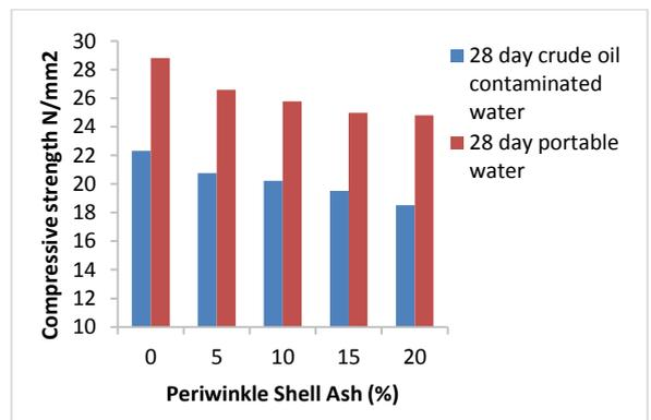
**Fig. 4:** Variation of compressive strength of periwinkle shell ash blended cement concrete cubes with periwinkle shell ash content cured for 28 days in portable water and crude oil contaminated water
