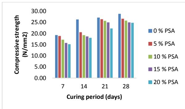
Fig. 5: Variation of compressive strength of periwinkle shell ash blended cement concrete cubes with curing period for specimen cured in portable water.
