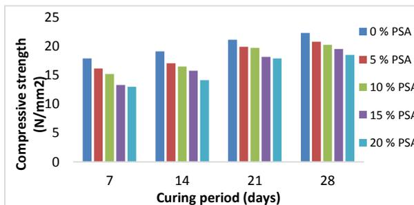
Fig. 6: Variation of compressive strength of periwinkle shell ash blended cement concrete cubes with curing period for specimen cured in crude oil contaminated water.
