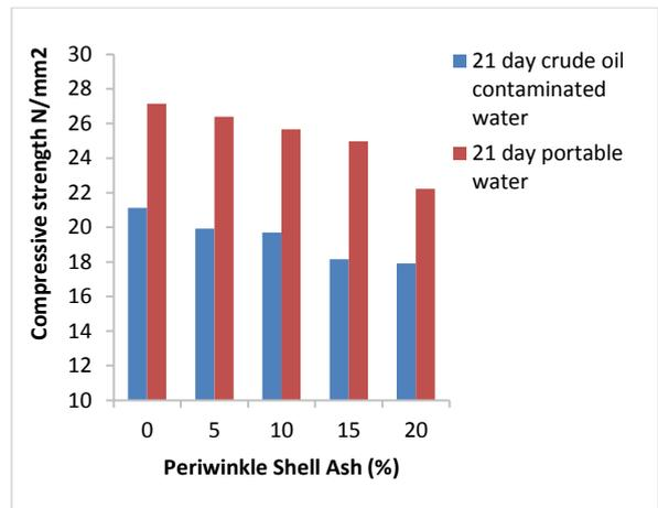
**Fig. 3:** Variation of compressive strength of periwinkle shell ash blended cement concrete cubes with periwinkle shell ash content cured for 21 days in portable water and crude oil contaminated water
