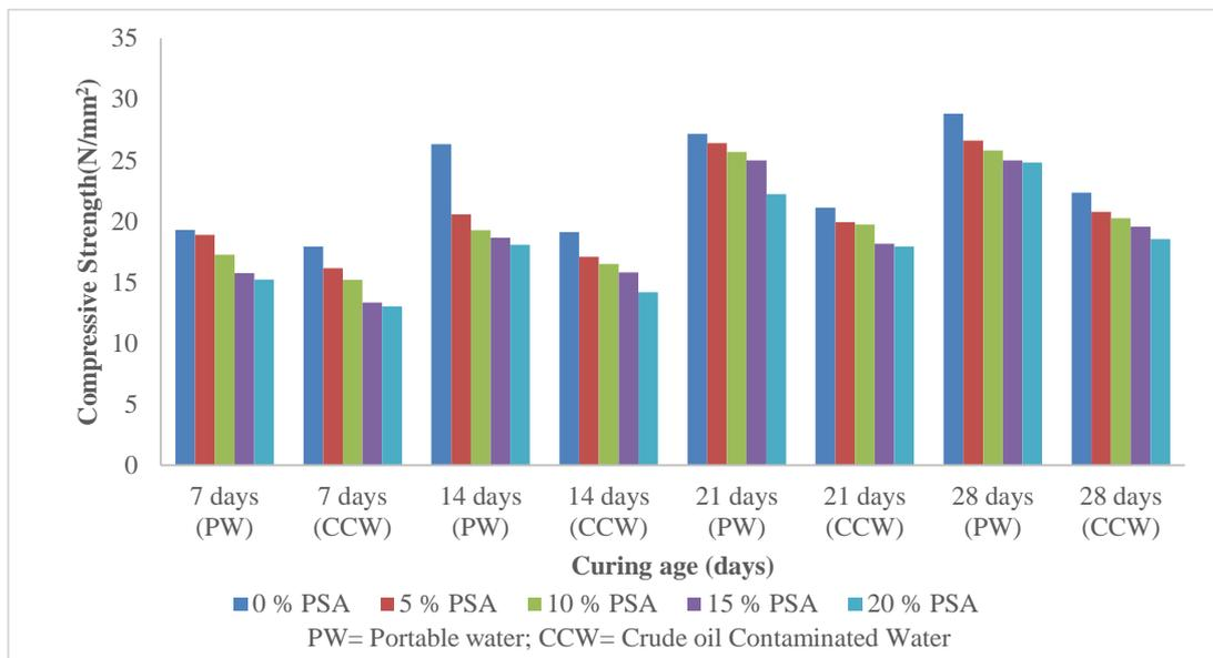
**Fig. 7:** Variation of compressive strength of periwinkle shell ash blended cement concrete cubes with curing age for specimens cured separately in portable water and crude oil contaminated water.
